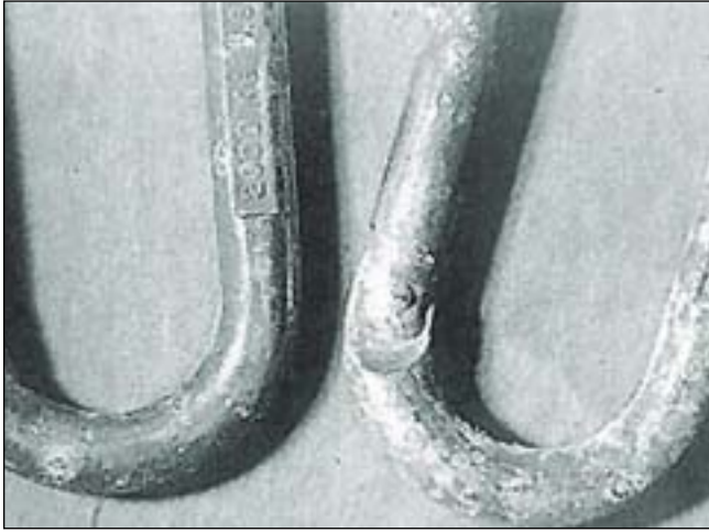
Fig 5 Test carabiners after nine months in a Virginia cave streamway. The one on the left was heat treated to the T7351 condition, while the one on the right received normal processing.
