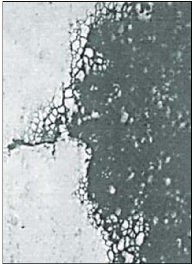
Fig. 2 Irregular surface of a pit with intergranular corrosion (approx 300x).
